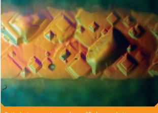
Optical microscopy image of a modified groove botton
