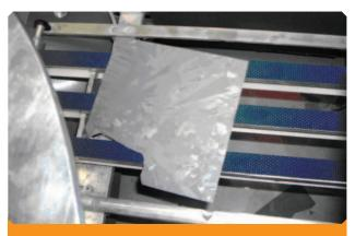
Broken wafer during thin wafer test run
